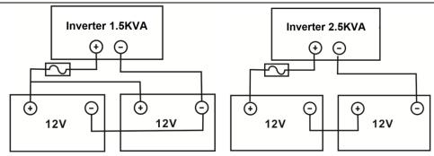
5. Insert the battery wires flatly into battery connectors of inverter and make sure the bolts are tightened with torque of 2 Nm in clockwise direction. Make sure polarity at both the battery and the inverter/charge is correctly connected and conductors are tightly screwed into the battery terminals.
