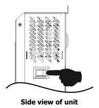
Once the unit has been properly installed and the batteries are connected well, simply press On/Off switch (located on the button of the case) to turn on the unit.
