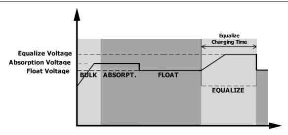
However, in Equalize stage, when battery equalized time is expired and battery voltage doesn't rise to battery equalization voltage point, the charge controller will extend the battery equalized time until battery voltage achieves battery equalization voltage. If battery voltage is still lower than battery equalization voltage when battery equalized timeout setting is over, the charge controller will stop equalization and return to float stage.
